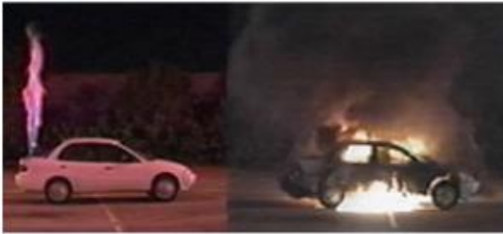
Fires from intentionally ignited fuel tanks containing hydrogen (left) v. gasoline (right)
